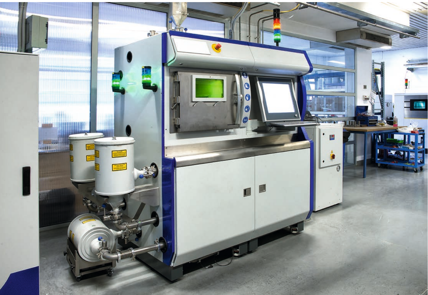
Metal 3D printer for direct metal laser sintering.
