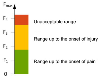
Figure 17. Example representation of the stress-strain relationship for one influencing variable (example here: crush forces on automatically closing doors)
